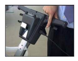
1. LIFT THE FLAP ON THE MACHINE HANDLE AND INSERT CHARGING LEAD.
