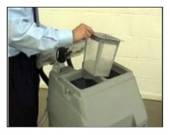
2. REMOVE THE FILTER FROM INSIDE THE TOP TANK.
