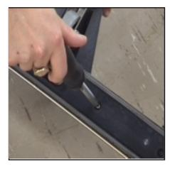
1. REMOVE THE SQUEEGEE TURN UPSIDE DOWN, AND REMOVE THE 4 SCREWS ALONG THE CENTRE OF THE TOOL.
