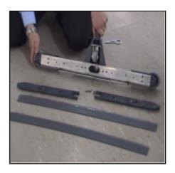
2. LIFT AND REMOVE THE 2 PLASTIC INSERTS AND DISCARD THE WORN BLADES.
