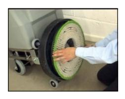
3. POSITION BRUSH ONTO THE GEARBOX WITH THE 3 INDENTATIONS ALLIGNING WITH THE 3 TABS. TURN ANTI-CLOCKWISE TO LOCK THE BRUSH IN PLACE.
