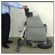
3. FOR TURNING IN TIGHT SPACES OR FOR LESS FLOOR PRESSURE, PUT THE HANDLE INTO A HIGHER POSITION.
