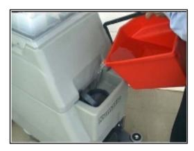
1. SIMPLY POUR WATER WITH A MIX OF YOUR CHOSEN DETERGENT INTO THE SPOUT ON THE FRONT OF THE BOTTOM TANK.
