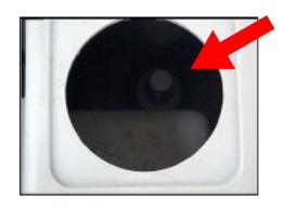
2. REMOVE THE FILTER FROM INSIDE THE BOTTOM TANK.
