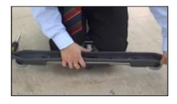
4. ALLIGN PLASTIC INSERTS AND APPLY PRESSURE UNTIL YOU FEEL THE BLADE GRIP INTO PLACE. REPLACE SCREWS AND PUT SQUEEGEE BACK ONTO MACHINE.
