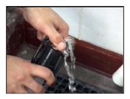
2. UNDO THE BALL VALVE ON HOSE.
