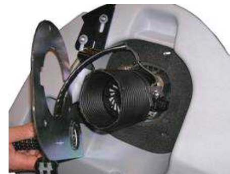
Insulated vacuum unit. 65 db(A) from 60" 1,5 metre distance
