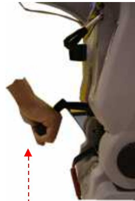
Squeegee is raised and lowered by handle
