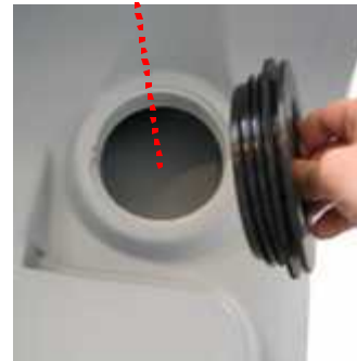
Rear solution tank inspection
