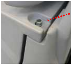
Unscrew bolt to tilt recovery tank sideways
