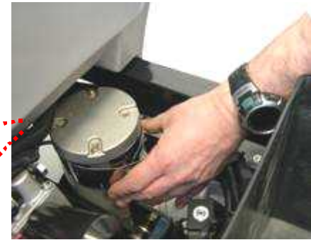
Brush motor carbon brushes replaced without tools
