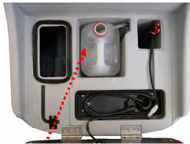
1.3 Gal (5 Ltr) chemical tank can be installed under the operators seat
