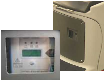
On board battery charger
