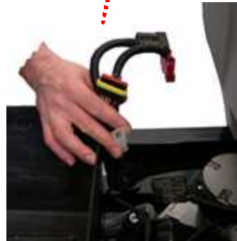
All major electrical areas easily disconnected by water proof plugs
