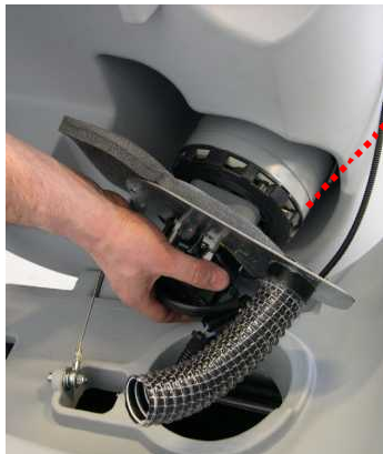
3 bolts to remove vacuum fan
