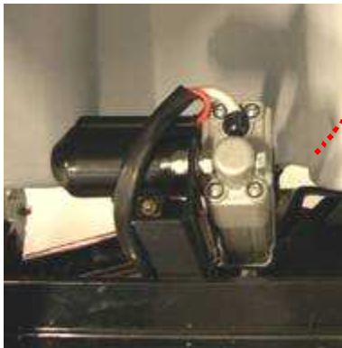
Easy to reach squeegee lifting actuator
