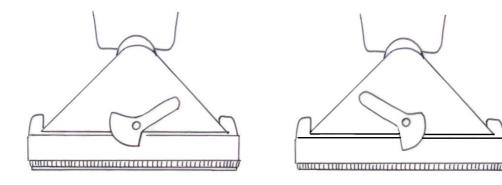
4. To activate the rotating brush switch the power to "on", the switch is located near the vacuum head.
