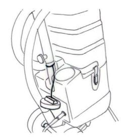
While filling the lower tank, pay attention to avoid overfilling the tank and to prevent water from spilling. Always keep in mind the dangers connected of spilling water on electrical components.
