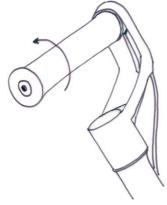
3. To clean carpets, rotate the lever on the vacuum head towards the right side. To clean hard floors, rotate it towards the left side.
