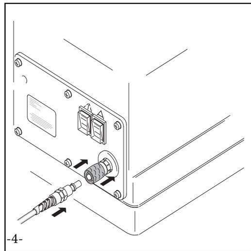
4. Connect the spray hose & gun to the machine. Verify the s/s tip is in the vertical position for optimal spray pattern. Plug the machine in, turn on and run the water through the unit. This helps remove any particles left in the unit, hose or gun during the manufacturing process
