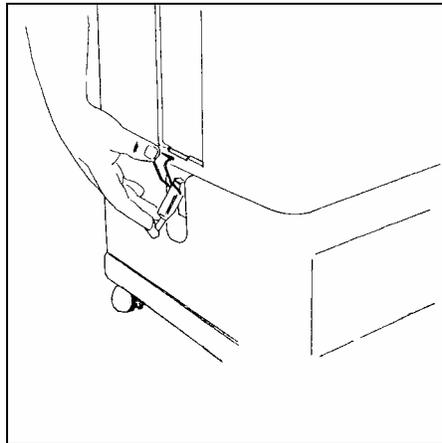
3. Fill the solution tank with 1 Gallon cold or warm water through the filling hole and then reconnect the tanks and fasten the springs.
