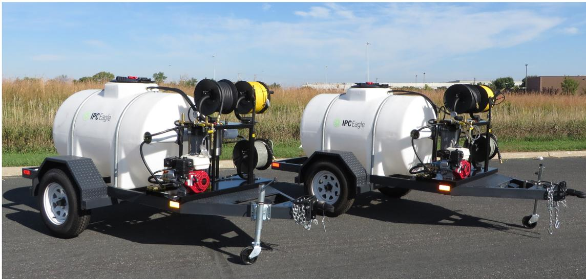
The **Hydro Station** is a compact and portable Pure Water Cleaning System. It can be mounted in an open or enclosed trailer. The Hydro Station has the unique ability to produce a high volume of pure water for multiple remote applications.
