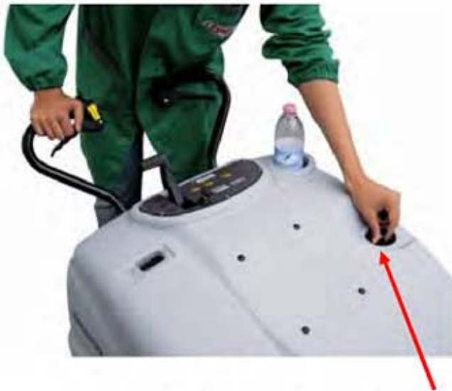
Brush pressure adjustment knob
