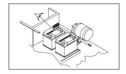
2 If the batteries are supplied without liquid (i.e. dry), they must be filled with sulphuric acid (density from 1.27 to 1.29 kg at 25℃), according to the instructions given in the next paragraph and in the battery handbook:
