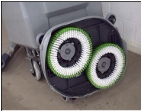
3. THE BRUSHES WILL NOW BE LOCKED IN PLACE AND READY FOR USE.
