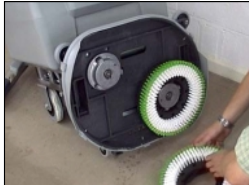
2. POSITION BRUSH ONTO THE GEARBOX WITH THE 3 INDENTATIONS ALLIGNING WITH THE 3 TABS. TURN ANTI-CLOCKWISE TO LOCK THE BRUSH IN PLACE.
